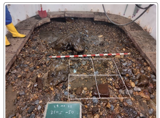
Fig. 1: Riverbed and quartzite blocks taken inside the diving bell of TGS Carl Straat
