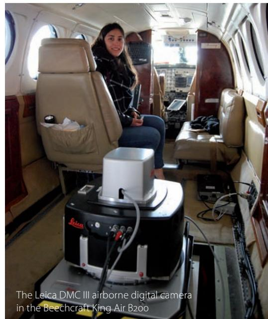
The Leica DMC III airborne digital camera in the Beechcraft King Air B200
