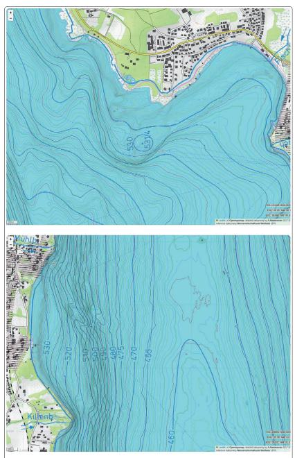
**Fig. 7:** Comparison of the isolines interpolated from the main dataset to the official 1979 sea chart in Herrsching/Rieder Eck (top) and in Utting (bottom)
