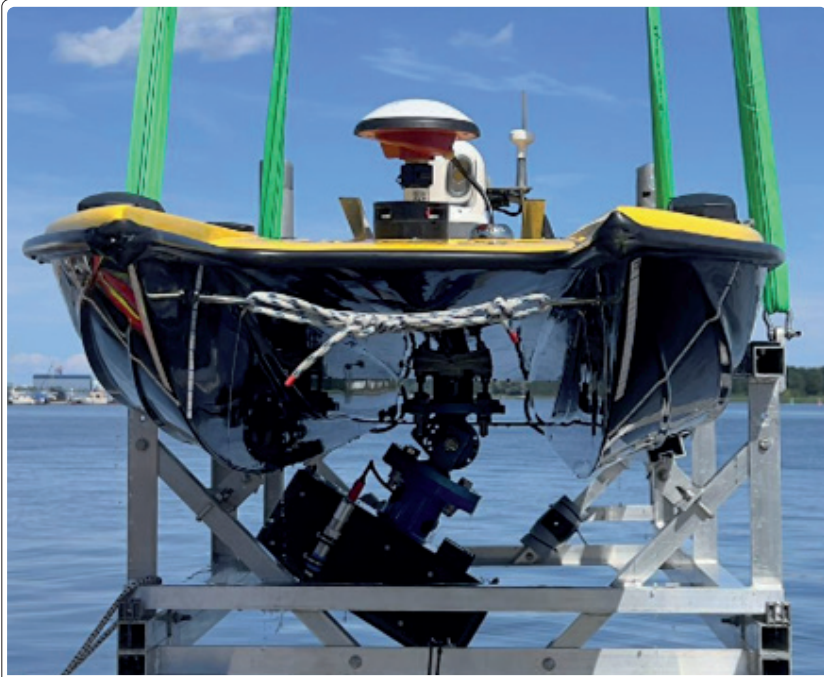
Fig. 1: The multibeam echo sounder was mounted on a tilted flange
