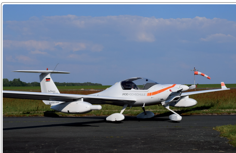
Fig. 1: The Jade University research aircraft »Jade One« with two external sensor containers
