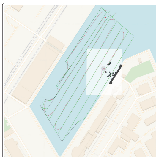
Fig. 3: Planned path by the ATB based on the defined polygon with detected obstacles (swimmers) in black
