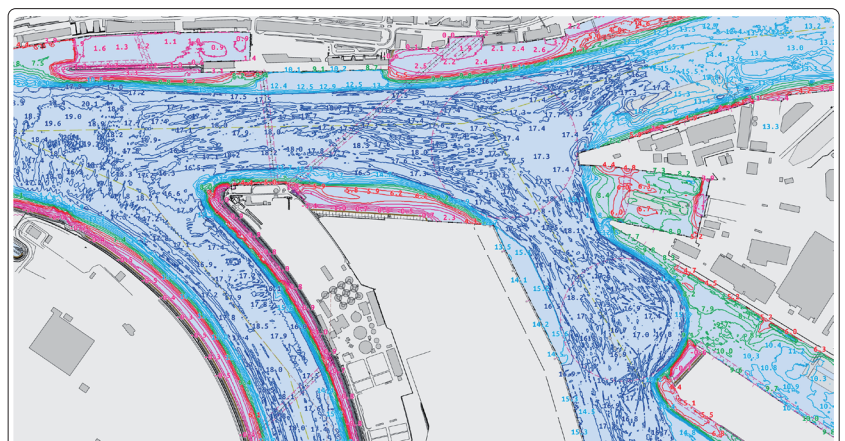
Fig. 6: Vector data visualisation in the Hydro Portal, showing soundings and contours for the harbour area
