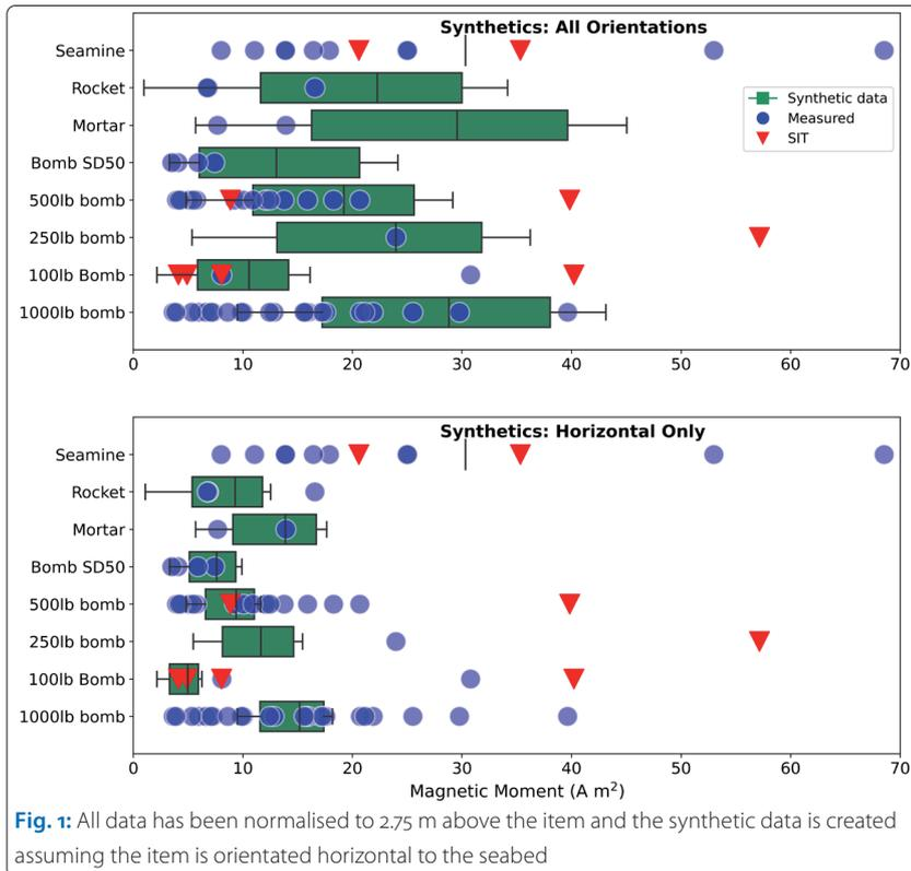
Fig. 1: All data has been normalised to 2.75 m above the item and the synthetic data is created assuming the item is orientated horizontal to the seabed
