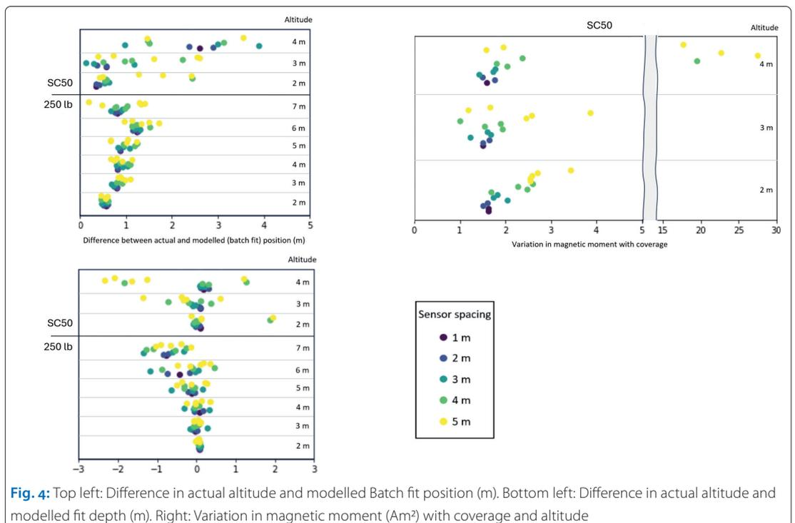
**Fig. 4:** Top left: Difference in actual altitude and modelled Batch fit position (m). Bottom left: Difference in actual altitude and modelled fit depth (m). Right: Variation in magnetic moment (Am<sup>2</sup>) with coverage and altitude
