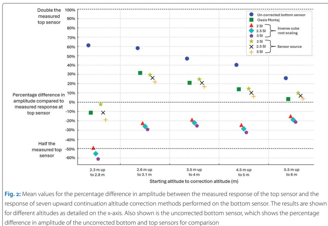
ent altitudes and extra care must be taken during background removal, target picking and modelling. Fig.2 highlights that the error when not correcting is greater than all the tested altitude correction approaches.
