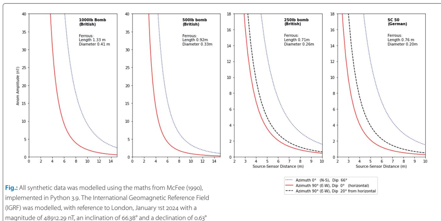
**Fig.:** All synthetic data was modelled using the maths from McFee (1990), implemented in Python 3.9. The International Geomagnetic Reference Field (IGRF) was modelled, with reference to London, January 1st 2024 with a magnitude of 48912.29 nT, an inclination of 66.38° and a declination of 0.63°
