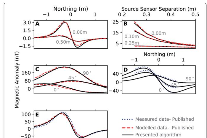
**Fig.:** As demonstrated in [Fact.Box.1](#) in practice it is possible for UXO to have lower responses than the synthetics, with munition degradation and lower sampling of responses not considered in the synthetics
