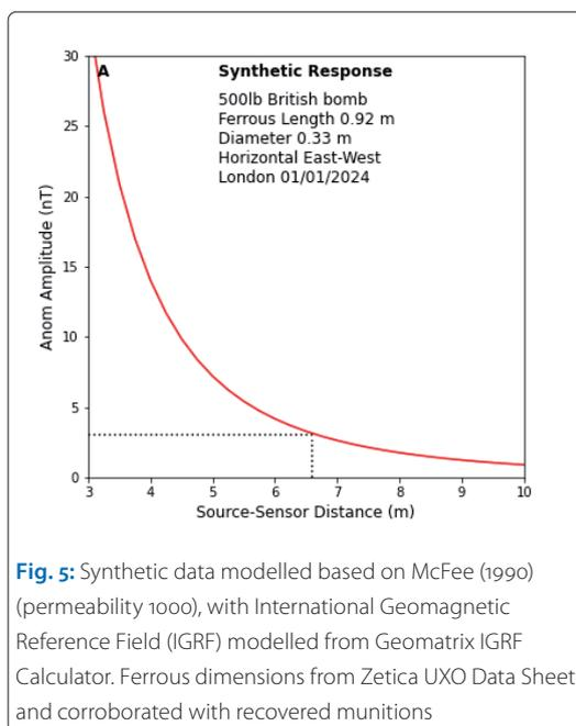
**Fig. 5:** Synthetic data modelled based on McFee (1990) (permeability 1000), with International Geomagnetic Reference Field (IGRF) modelled from Geomatrix IGRF Calculator. Ferrous dimensions from Zetica UXO Data Sheet and corroborated with recovered munitions
