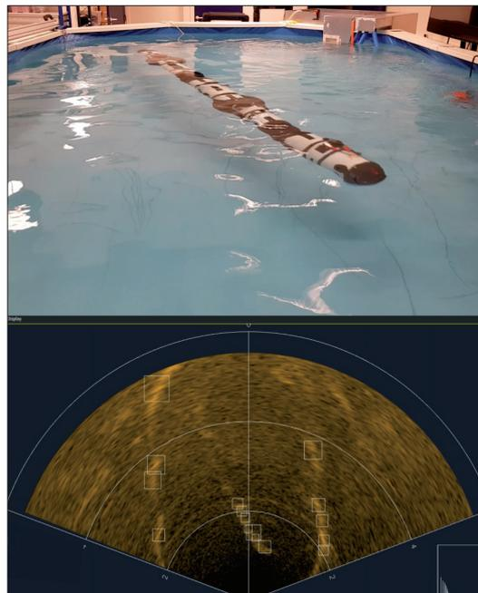
Fig. 8: In the bottom screen, you can see the FLS view of the pool with the Eelume AUV in it – the squares show where NaviSuite software uses machine learning to automatically register objects, namely the AUV in the centre, as well as interference from the sides of the pool
