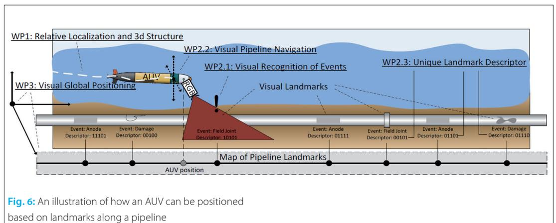
**Fig. 6:** An illustration of how an AUV can be positioned based on landmarks along a pipeline
