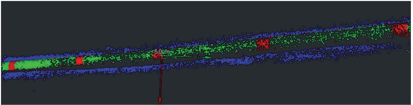
**Fig. 9:** A sparse point cloud of a pipeline, created using VSLAM and coloured using analysis by NaviSuite Deep Learning – the green points are the pipeline, the red are anodes and blue shows the sea bottom
