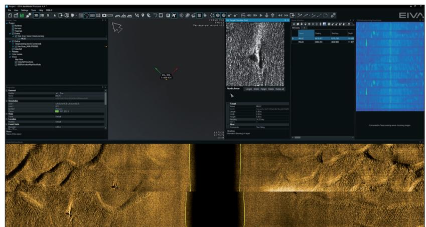
Fig. 3: The Automatic Target Recognition (ATR) tool uses a variety of NaviModel functions to identify objects – in addition to DTMs, it can be used on side-scan sonar data, as shown here, where two objects have been automatically registered as events, as shown in the event window (upper right)
