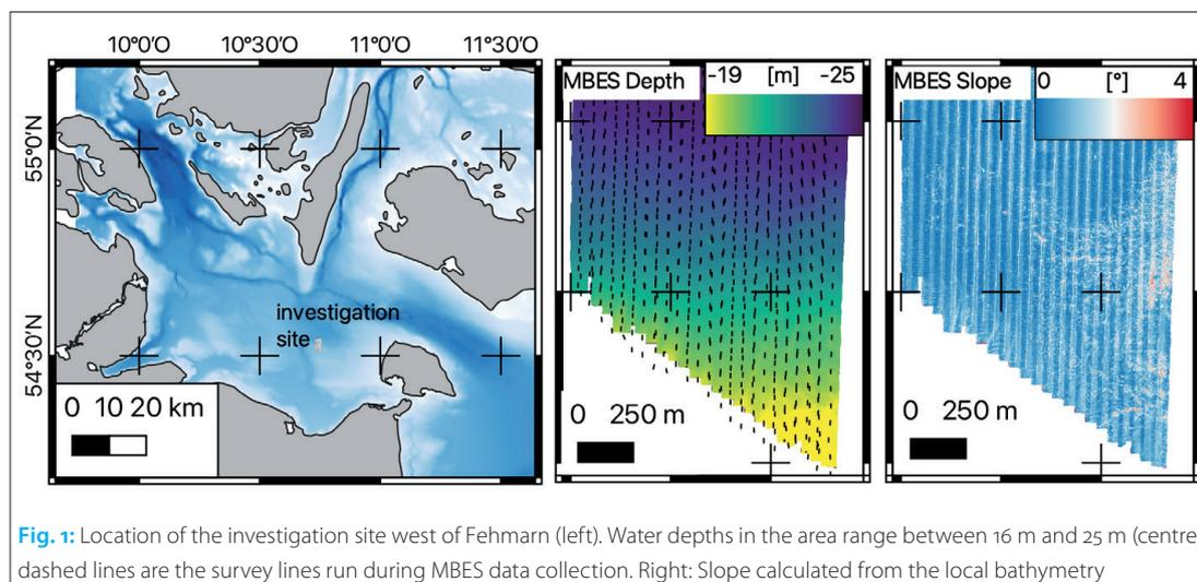
**Fig. 1:** Location of the investigation site west of Fehmarn (left). Water depths in the area range between 16 m and 25 m (centre), dashed lines are the survey lines run during MBES data collection. Right: Slope calculated from the local bathymetry
