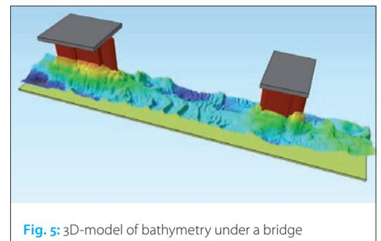
Fig. 5: 3D-model of bathymetry under a bridge
