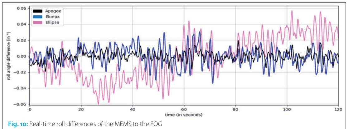
Fig. 10: Real-time roll differences of the MEMS to the FOG
