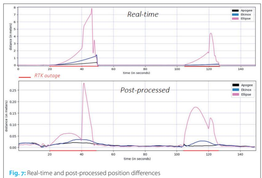
Fig. 7: Real-time and post-processed position differences
