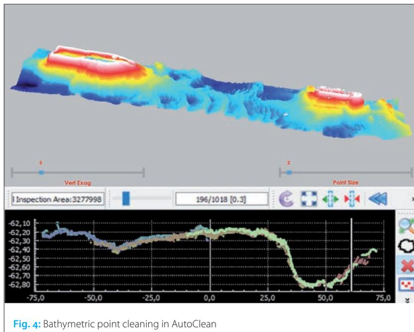
Fig. 4: Bathymetric point cleaning in AutoClean
