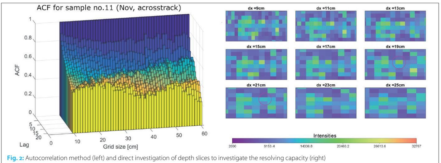
Fig. 2: Autocorrelation method (left) and direct investigation of depth slices to investigate the resolving capacity (right)
