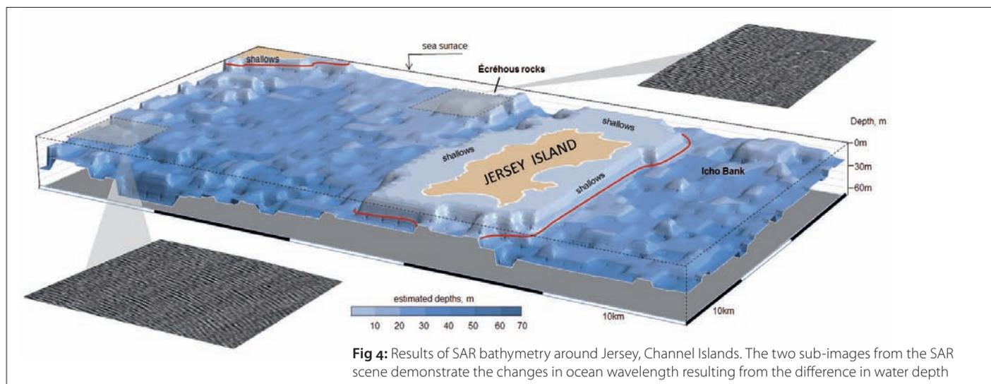
**Fig 4:** Results of SAR bathymetry around Jersey, Channel Islands. The two sub-images from the SAR scene demonstrate the changes in ocean wavelength resulting from the difference in water depth
