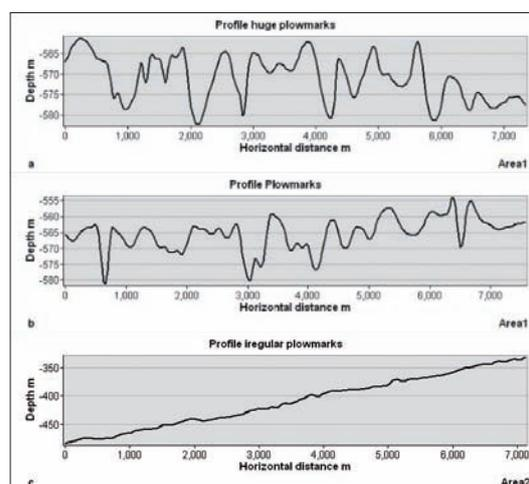
**Fig. 4a:** Cross-section of huge plough marks DD' on the northeastern part of Area 1. **b:** Cross-section of fresh-looking plough marks EE' on Area 1. **c:** Cross-section of irregular plough marks FF' on Area 2
