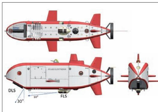
Fig. 2: IMGAM vehicle and mission specific systems
