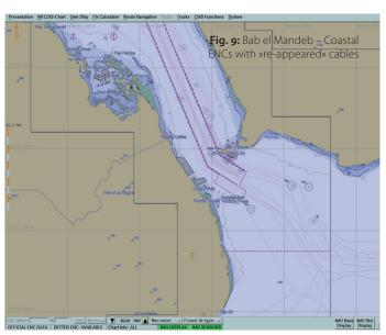
However, only a small area is shown now – an overview of where the cables come from and run to is not provided at this display scale.
