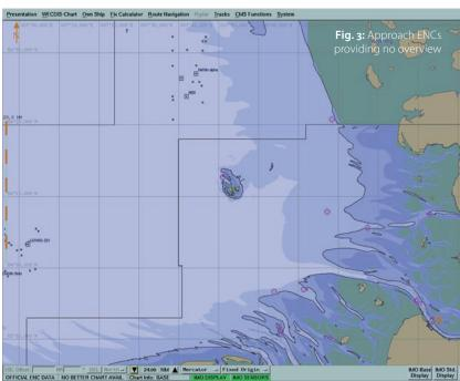
display range of 96 nm (with the »display range« being the range from the centre of the display to its top). It can be clearly seen that the entire coastal waters are covered by a greenish area. Greenish stands for »intertidal areas«, sea areas that fall dry at low water.
