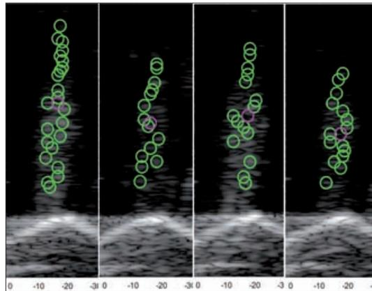
**Fig. 8:** Automatic cyclical steering of the transmitted swath (advanced transmission beam steering)
