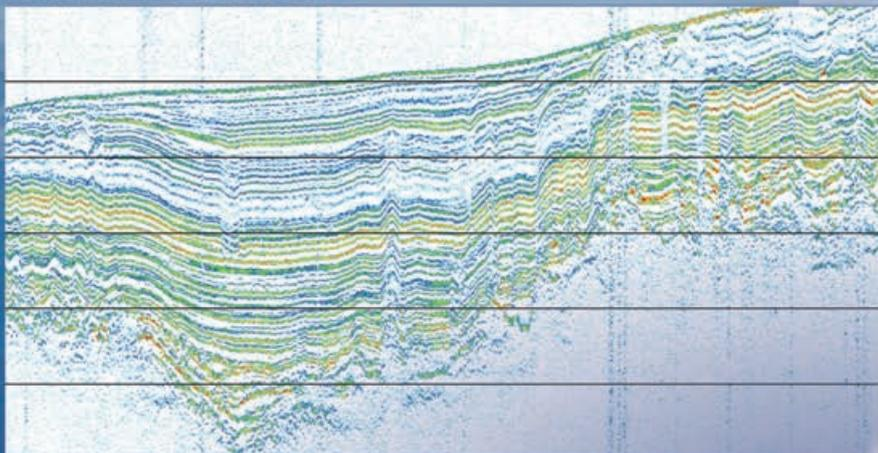
Frequency 8kHz, pulse length 375 μs (SES-2000 light), Baltic Sea
