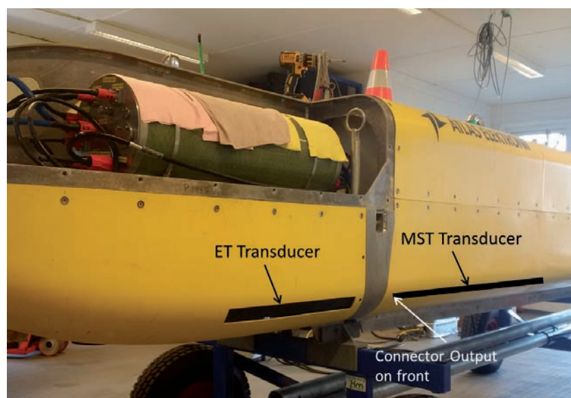
Fig. 1: Mounting of the sonars on the AUV
